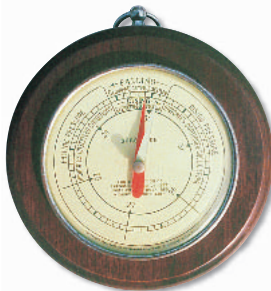
Figure 10 A barometer measures atmospheric pressure. The red pointer points to the current pressure. Watch how atmospheric pressure changes over time when you line up the white pointer to the one indicating the current pressure each day.
