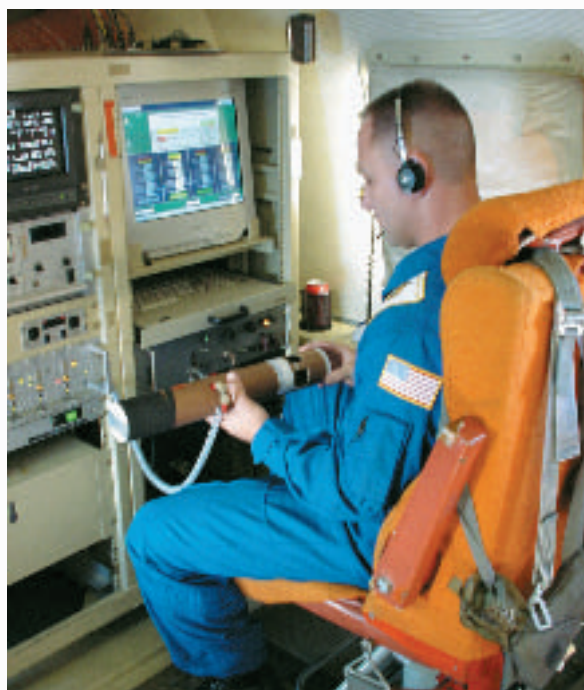
Figure 3 Dropsondes released from aircraft collect information as they fall through a hurricane.
